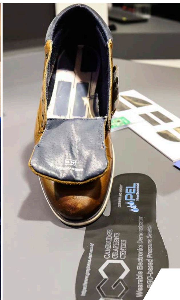
Pressure sensing insoles made of lightweight graphene-embedded foam could be integrated into any type of shoe.
